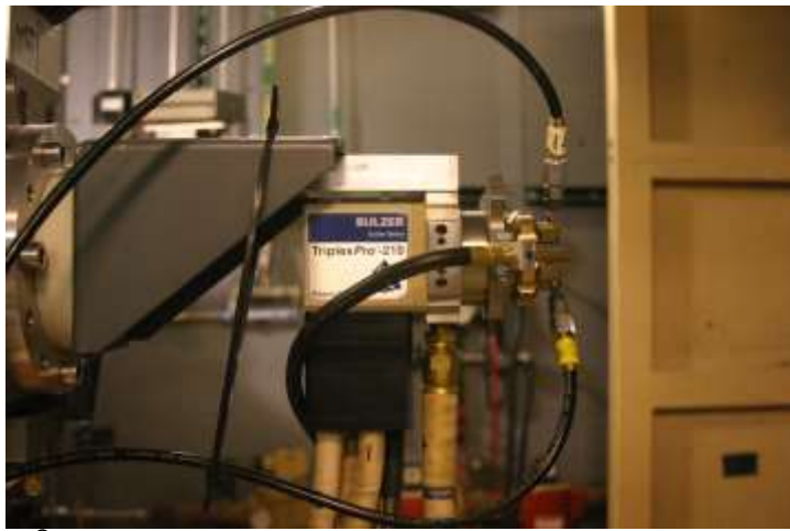
Figure 1: TriplexPro®-210 air plasma spray torch (Sulzer-Metco, Inc. Westbury, NY) used to prepare molybdenum coatings at Sandia's Thermal Spray Research Laboratory.
