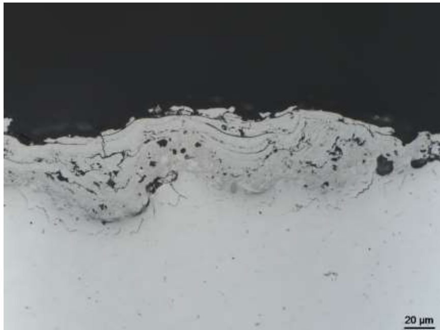
Figure 21: Polished cross section showing sprayed Mo (70μm powder size) coating on the Bi 2 Te 3 substrate. This higher magnification image showed signs of possible Mo-Bi 2 Te 3 mechanical interaction at the wavy coating/substrate interface. Subsequent layers of Mo showed the elongated grains “splats” containing columnar structures, typical of coatings prepared using APS. Note the cracks immediately below the interface, along the grain boundaries of the Bi 2 Te 3 substrate.
