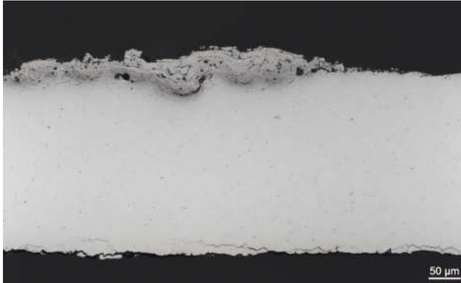
Figure 20: Polished cross section showing the Mo (70μm powder size) coating on the Bi 2 Te 3 substrate. The transition between the sprayed and masked regions can be seen at the right side of the image. Notice that the uncoated substrate on the right-hand side is much smoother (more planar) compared to the substrate beneath the Mo sprayed coating on the left-hand side of the image.
