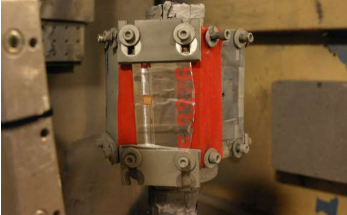
Figure 7: Fully masked \text{Al}_2\text{O}_3 substrate (with silicone and aluminum tapes) attached to a rotary fixture ready to be plasma sprayed with Molybdenum. The air knife seen in the left foreground of this image is positioned \sim 90^\circ from the spray plume. This allowed the coated part to rapidly pass through the plasma and then immediately through the cooling air jet as the fixture rotated.
