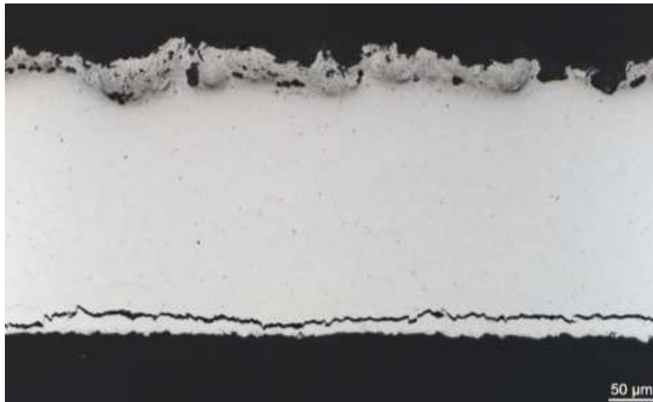
Figure 19: Polished cross section of the sprayed Mo (70μm powder size) on \text{Bi}_2\text{Te}_3 substrate. The coating/substrate interface appeared wavy and contained voids. Note that cracks are present immediately below the coating-substrate interface, along the grain boundaries the \text{Bi}_2\text{Te}_3 .
