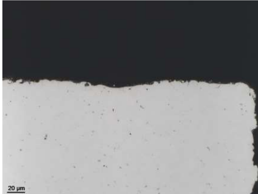
Figure 18: Polished cross section of the unsprayed \text{Bi}_2\text{Te}_3 substrate. This higher magnification picture still showed signs of pre-existing voids and cracks right below the substrate surface, along the grain boundaries.
