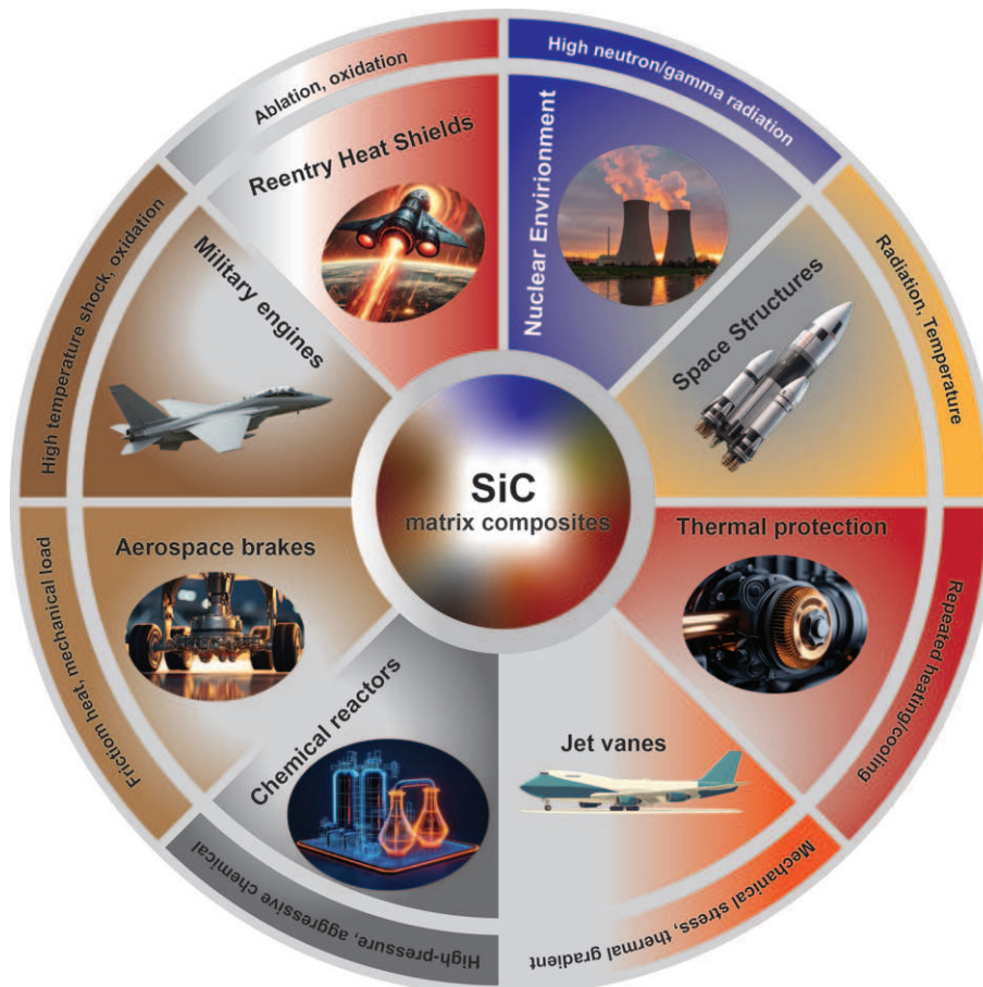
Fig. 1: Extreme environments and representative application fields of SiC-matrix composites. Image source: Adobe Stock.
